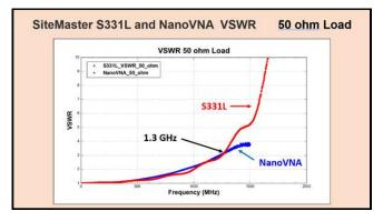
The results of this extensive testing are too numerous to document here, however in summary the nanoVNA compared favorably to the S331L for frequencies less than 900 MHZ. For frequencies above 900 MHz, the nanoVNA exhibited increased variation when referenced to the S331L data results.
