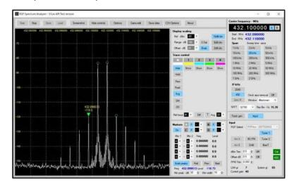
The illustration depicts intermodulation distortion (IMD) measurements for a 70 cm amplifier I had constructed.
