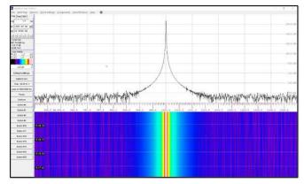
Utilizing a GPSDO controlled SDR combined with Spectrum Lab Software (Author: Wolfgang "Wolf" Buescher DL4YHF) provides remarkable frequency determination. This method, or similar technology, is frequently used for the ARRL FMT contest. With careful procedures frequency accuracy may approach 1X10<sup>-12</sup> (0.000001 ppm).
