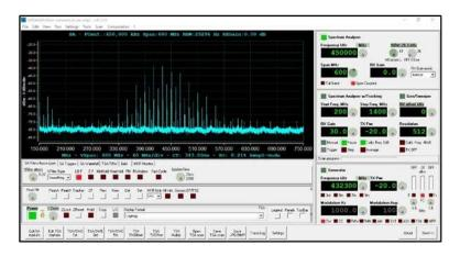
Alternatively, a low-cost RF noise source may be used as a signal source and frequency response of the 70 cm bandpass filter determined. Once again, all data and measurements results may be saved to a computer file for additional inspection or future review.
