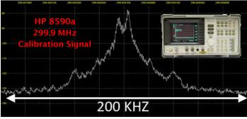
I thought it interesting to conduct a spectral comparison of a RF signal generated by the nanoVNA versus the nominal 300 MHz calibration signal generated by the legacy HP 8590a technology.
