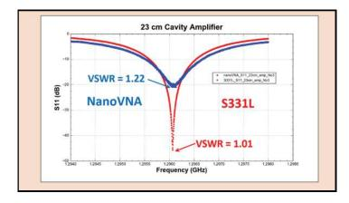
As previously described, when conducting measurements above 900 MHZ some differences were noted between nanoVNA and \$331l results. The data shows \$11 measurements conducted on a 23 cm 1296 MHz) resonant cavity. It is likely this difference would be resolved using a more current nanoVNA model versus the original model H that I used for these tests.
