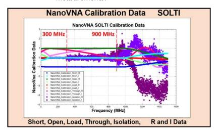
This calibration data example shows calibration values for the nanoVNA obtained through this procedure.
