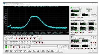
The Spectrum Analyzer plus Tracking Generator function is particularly useful for measurement of RF amplifiers, RF directional couplers, RF filters, RF attenuators.
