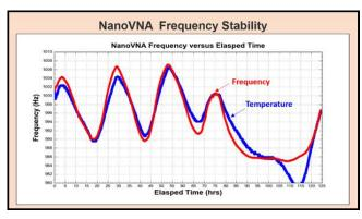
GPSDO controlled SDR receiver. Data obtained over a 5-day interval shows frequency variation of approximately 20 Hz, (0.05 ppm). NanoVNA absolute accuracy averaged 50 Hz (0.1 PPM).
