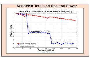
Total and frequency spectral analysis methods were applied to measure RF power levels at specific frequency values. This data shows some 16-decibel reduction in power for frequencies greater than 900 MHz compared to the sub 300 MHz values. This reduction in signal level at elevated frequencies places some limitations on measurement accuracy principally due to reduction of signal to noise values.
