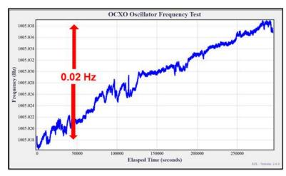
In this example 0.02 Hz (~ 0.002 ppm) frequency drift was noted over an 8 day test period.
