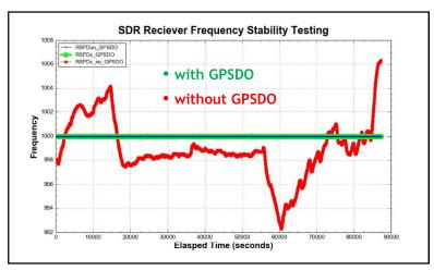
This data collected sequentially over a total period of two days. Inspection of this indicates the approximately 12 Hz frequency drift was reduced to essentially Zero with the GPSDO provding the frequency reference clock oscillator for the SDR.
