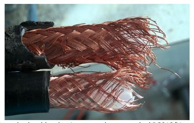
To be perfectly clear - both cables that I compared were marked RG213/U.
