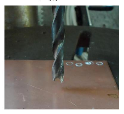
The PCB **must** be clamped down to the drill press table. Set the drill press stop using a piece of steel slightly thinner than the PCB stock.
