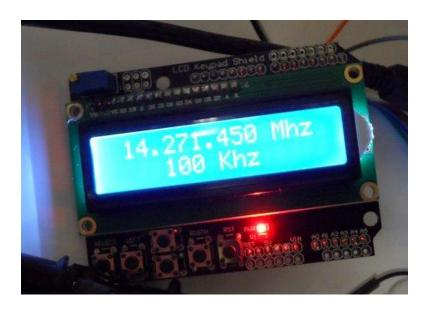
I soldered a replacement oscillator into the first DDS module and it came to life. The oscillator modules are recommended for dongle down-converter receivers, so I will have more projects to work on.
